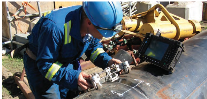
A technician scans pipe with ultrasonic imaging technology.
