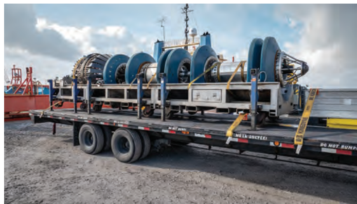
Pipeline inspection tools travel inside the pipe scanning with technology like an MRI or ultrasound.
